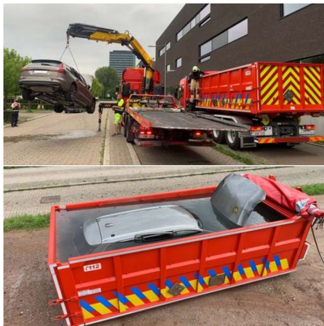
Figure 7. Use of a container for submerging electric vehicles in water.
