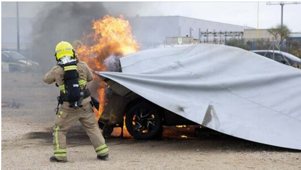
Figure 6. Use of a fire-resistant blanket in fire suppression
